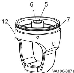
Figure 33: Remove Yoke O-ring and Guide Bearing
